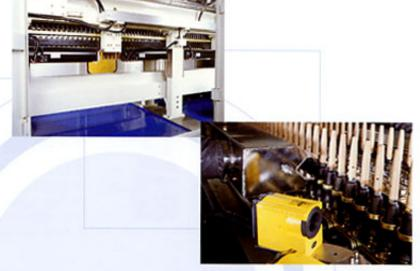
▲ Fast cooling down design on preform body----with a new adjustable airknife, preform body and adaptor can be more efficiently cooled down respectively.
