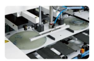
The auto folding device can fold up the pile of the bags very shipshape.
