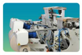
Independent pneumatic unwind system film roll E.P.C. turning adjustment and independ tension control.
