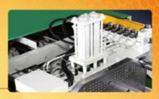
The machine can achieve dualpurpose by operating with rotary table and spindle alternatively.
