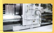
The balance design of rotary table effectivly keeps balance on mold to avoid table leaning forward and hold the mold stable without damaging guide pins.
