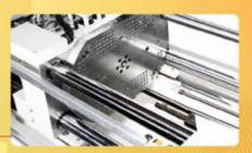
The balance design of moving platen keeps the precision of levelness in operation by adjusting rotary table according to mold weight to protect guide pins and ensure mold closing precisely.
