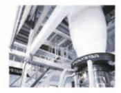
In some markets where shopping and T-shirt bag production has become extremely competitive, film producers are replacing their existing monolayer extruders with ABA 3 layer blown film machines to reduce production cost.
